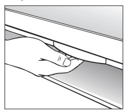
At the end of programmes with a drying phase (see "Programme chart") the door will open automatically a little in order to help the drying process.
